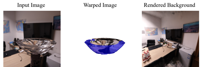
Fig. 2. The recovered background image and warped image on real data. Based on our experience, we roughly annotated some total internal reflection regions with blue masks to facilitate comparative analysis of the remaining areas.
